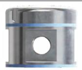
Construction: Nickel Plated Brass Round box consisting of a base and lid. Supplied with blue high visibility polyester elastomer lid and base seals. Available with either 2 or 4 holes, other versions available on request. 2 Fixing holes are provided, together with component Mounting holes to help with installation. Slots in the lid allow for secure tightening of the lid and aids opening for maintenance or upgrade. Design offers high Ingress Protection.
